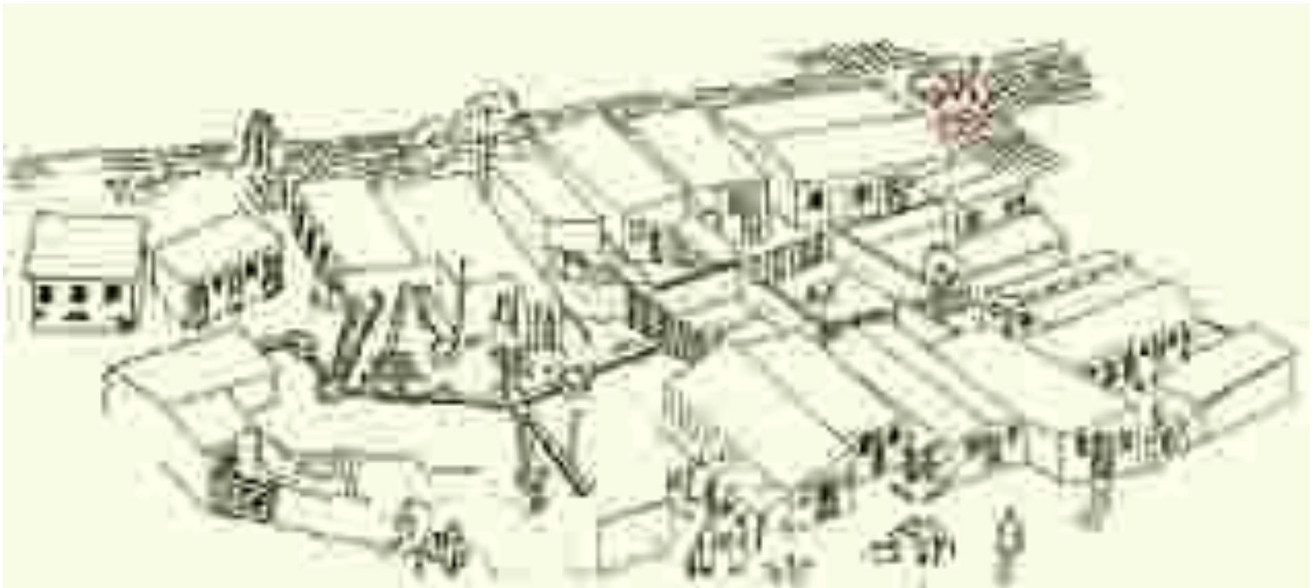
Figure 2-5: Typical Simplified Sewerage system layout aerial view
